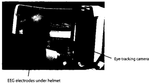
*Figure 1. Integration of eye-tracking and Electroencephalography (EEG) tools during operator-system interaction. Eye-tracking and EEG provide continuous, objective measurements of operator performance.*
