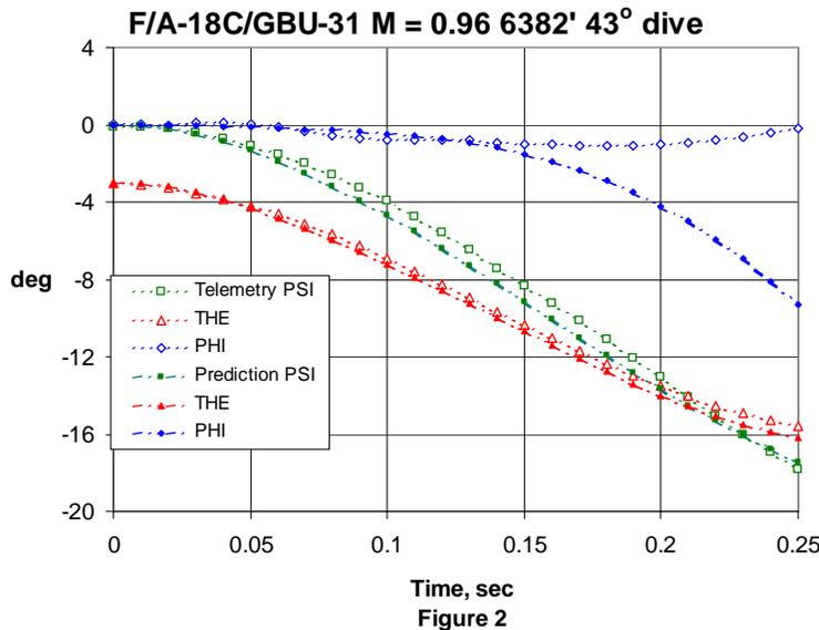
Recently, the GBU-31, GBU-32 and GBU-38 (GBU refers to Glide Bomb Unit) stores certification programs were successfully completed using one value of  $x$ ,  $y$ , and roll angle, and three values of yaw and pitch angles (7 grids). As may be seen in Figure 2, excellent correlation was achieved between the predictions and test data.
