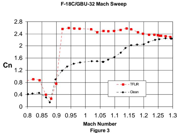
in tunnel Mach number in the transonic range (i.e.  $M=0.02$ ). As may be seen in Figure 3, the yawing moment for the GBU-32 store changes by more than 100% between  $M = 0.90$  and  $0.92$ . Furthermore, aircraft configuration changes have a significant impact on the store aerodynamics. The large yawing moment effect of the Targeting Forward Looking Infrared (TFLIR) can be easily seen in Figure 3.
