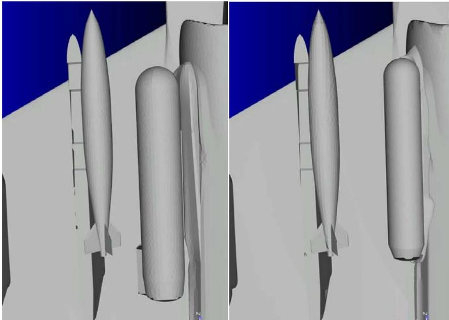
**Figure 5. Relative Distance Between Litening Pod (left) or ATFLIR (right) and MK-82 Store.**
