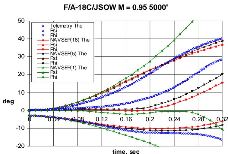
**Figure 5 F-18C/JSOW Grid Effects on Trajectory Prediction**
