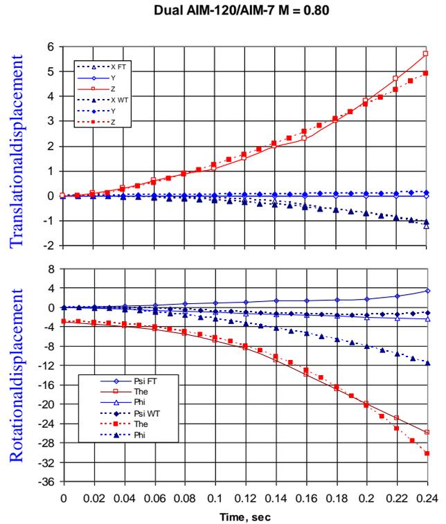
Fig. 9 Comparisons of flight-telemetry data with the predicted trajectory of a dual AIM-120 – Translational- and rotational-displacement time histories
