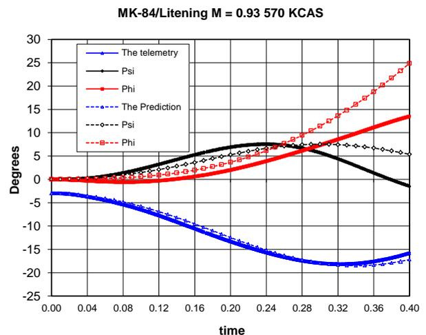
Fig. 8 Comparisons of MK-84 trajectory predictions with flight-test data
