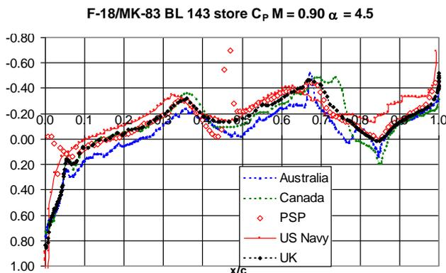
Fig. 4 Comparison of PSP test data with CFD predictions
