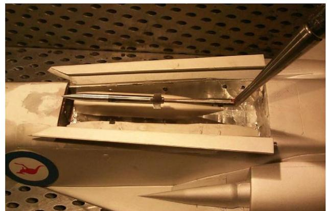
Fig. 6 Aft sting arrangement for SSB in F-111 bomb bay
