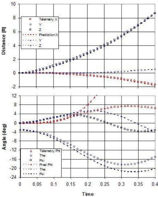
Fig. 11 Comparisons of Flight-Telemetry Data with the Predicted Trajectory of an Mk83
