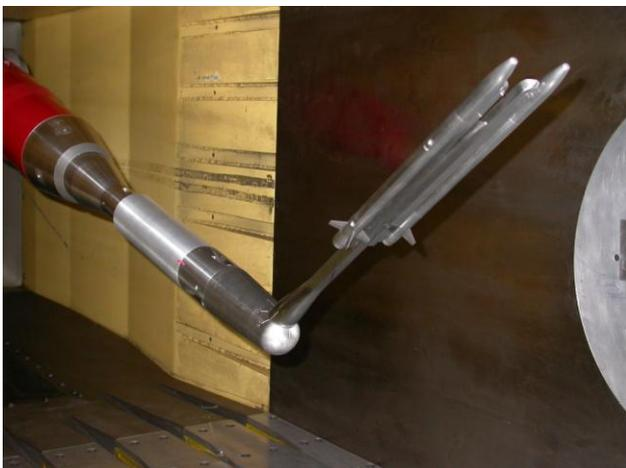
Fig. 10 Dual AIM-120 and LAU-127 launcher mounting system in the DSTO Transonic Wind Tunnel
