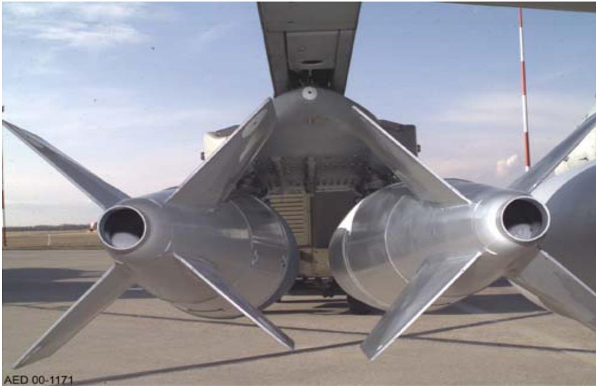
**Figure 9: CF-18/MK-83 Carriage Position**
