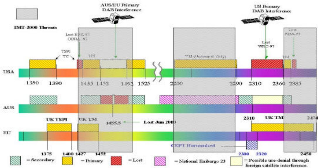
Figure 3. Telemetry Band Congestion
