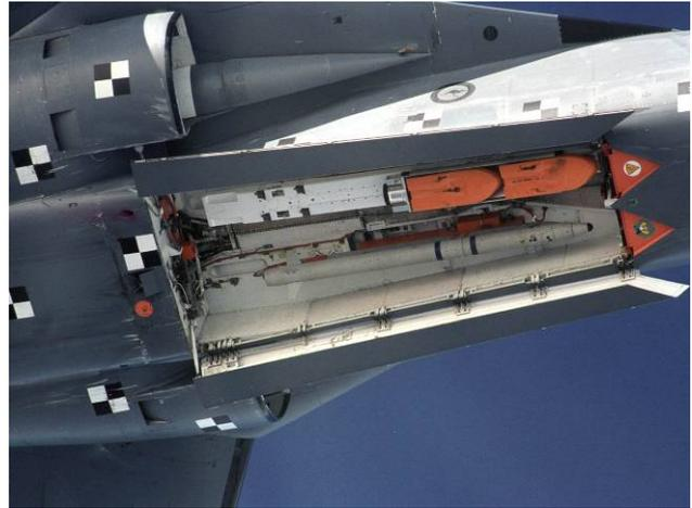
Fig. 5 F-111 Weapon bay with PLOCAAS in-flight.
