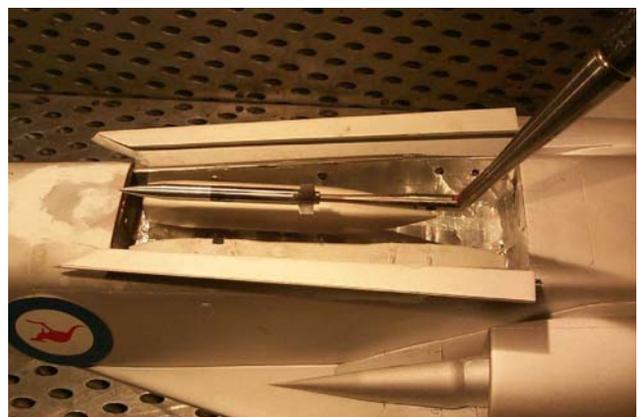
Fig. 4 Aft-sting arrangement for SSB in F-111 bomb bay similarly from [4]
